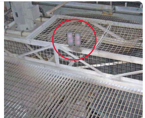
Lubrication system: 2 x perma STAR VARIO 120 cm 3
