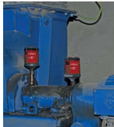
Lubrication system: 2 x perma STAR VARIO 250 cm 3
