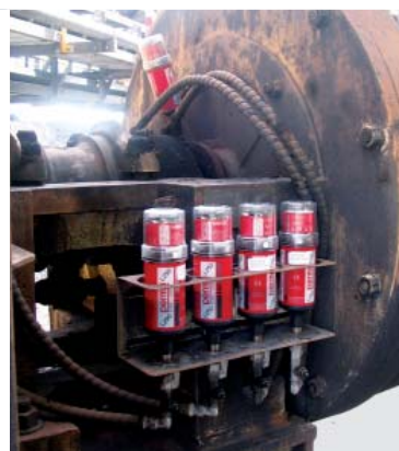
Lubrication system: 5 perma STAR VARIO 250 cm 3 each
