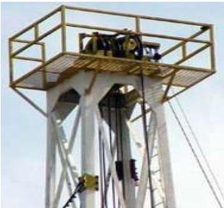
The LUBECORE system used to lubricate the Crown bearings represents one of the most cost effective applications on the rig. Saving both time and money when safety is the priority.
