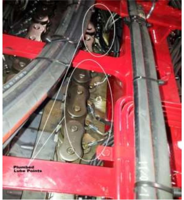
Distribution blocks and lines are available and all rated for high pressures in order for the **LUBECORE** pump to be able to deliver grease long distances to difficult to access lube points.
