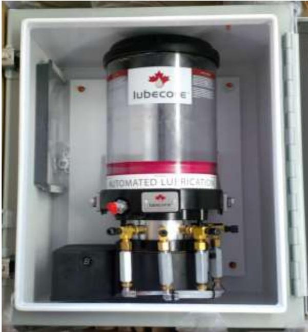
(above left) The LUBECORE system is flexible to facilitate multiple lube points depending on the application requirements. Has the capability of automatic re-lubrication of multiple bearings located on the crown of a drilling rig 150' up all from the drill floor. Utilizing the LUBECORE system all bearings receive controlled, uncontaminated lubrication on a consistent basis. Most units are mounted directly on the crown.
